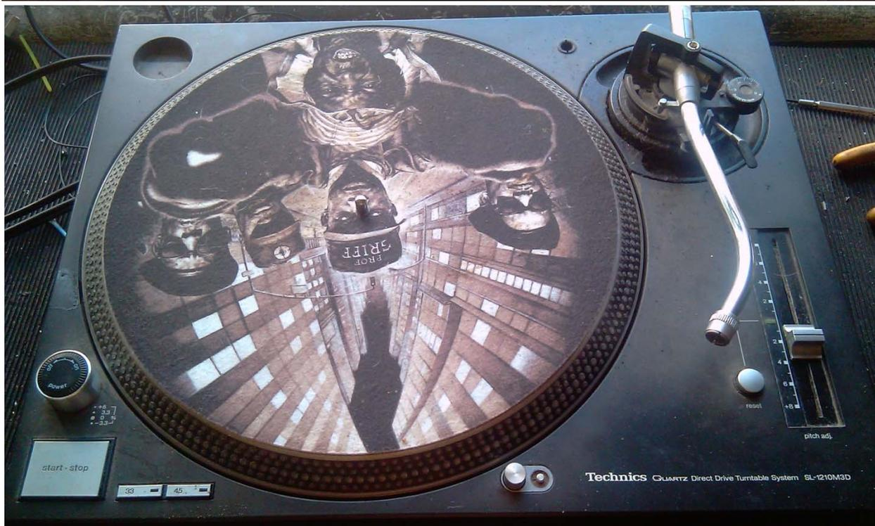
Strobe Leds will be changed if there dim \$9 will be charged for the parts but no extra labour charge. You can also request different colored Leds. Full set which includes 33/45 / Strobe / Pitch / and Target \$18, colors include: UV - White- Blue- Green - Yellow – Red or any combination.
